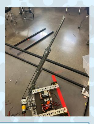
The hook is currently too large, which causes it to interfere with the claw, preventing the arm from fully retracting and staying out of the way. This also affects the functionality of the hooks, making them unable to operate correctly. Additionally, the wires need proper connections to ensure they function as intended.
