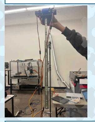
The height of the arm when fully extended is approximately 260 mm, but it is still not sufficient to reach the tallest basket. To address this, we plan to extend the arm slightly in order to ensure it can reach the highest basket.
