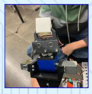
A rotating arm that picks up blocks using a bevel gear system relies on a motor to drive the motion through gears arranged at an angle. The bevel gears transfer rotational motion from the motor's shaft to the arm, which is mounted on another shaft. In this setup, the bevel gear system physically transfers the rotational motion from the motor to the arm. While the bevel gears affect the speed and torque of the arm, they don't require changes to the code, as the system operates mechanically.
